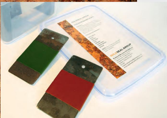
**OBJECTIVE:** To provide colour samples of Goldseal Hot Spray and ready for use steel panels in Industrial Hot Spray Red, to hang in corrosive environments for performance monitoring and easy inspection.
